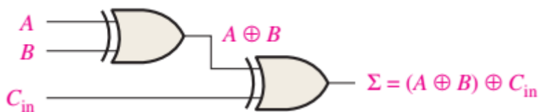
(a) Logic required to form the sum of three bits
